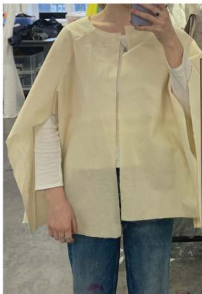
ADAPTING A RAGLAN SLEEVE PATTERN TO CREATE AN OPENING FOR THE ARM
