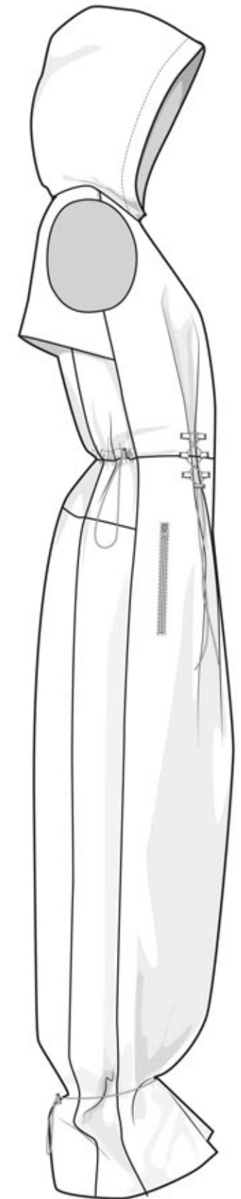
INTERNAL STRAIGHT SEAMS SEALED WITH 20MM WATERPROOF TAPE
