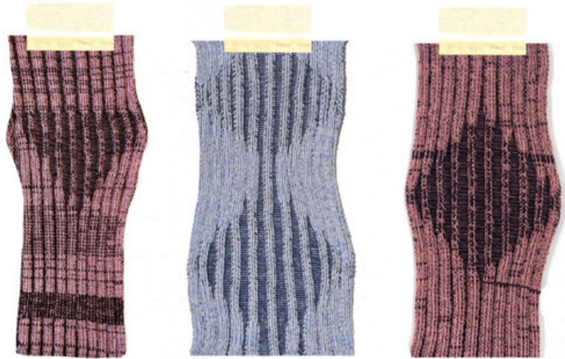
ALTERING THE SIZE OF THE PLATED RIB TO CREATE CURVED PATTERNS
