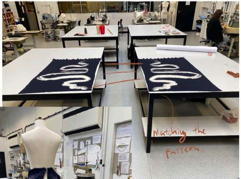
Front & Back panel are joined, try to reduce as much waste, low waste pattern cutting.
