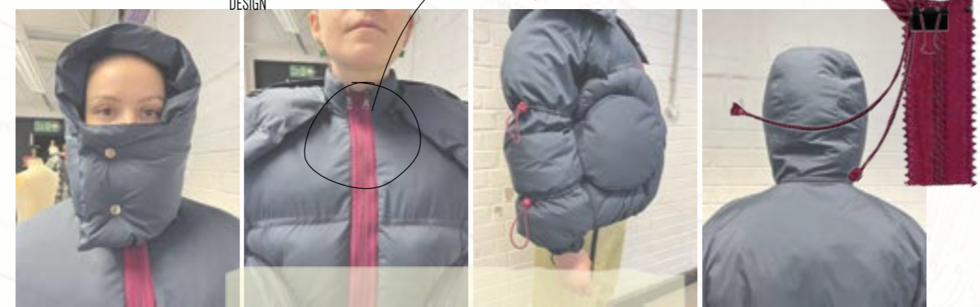
CREATED A DOUBLE CENTRE FRONT ZIP USING THE ULTRA SONIC WELDER MACHINE. CREATED A STRONG BOND FOR ZIP SUITABLE FOR A FUNCTIONAL GARMENT, AS WELL AS INNOVATIVE FEATURE ON ZIP.
