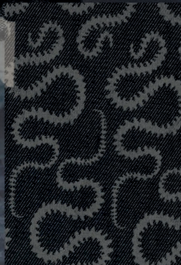
Laser engraving on cotton denim.
