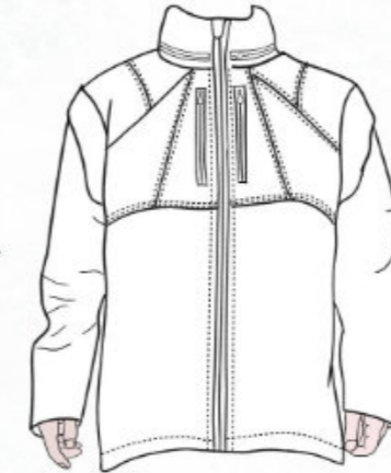
WHITE AQUAGUARD CLOSED (X3) 18CM WHITE AQUAGUARD CLOSED (X2) 56.2CM WHITE AQUAGUARD CLOSED (X1) COLLAR TOTAL = 57.2 (TO EDGE OF SEAM ALLOWANCE) MEASURE AT HOME TAKE OFF 1.5CM EACH SIDE SO 54.2CM WHITE CHUNKY DOUBLE-ENDED OPEN ZIP (X1) 7.5CM
