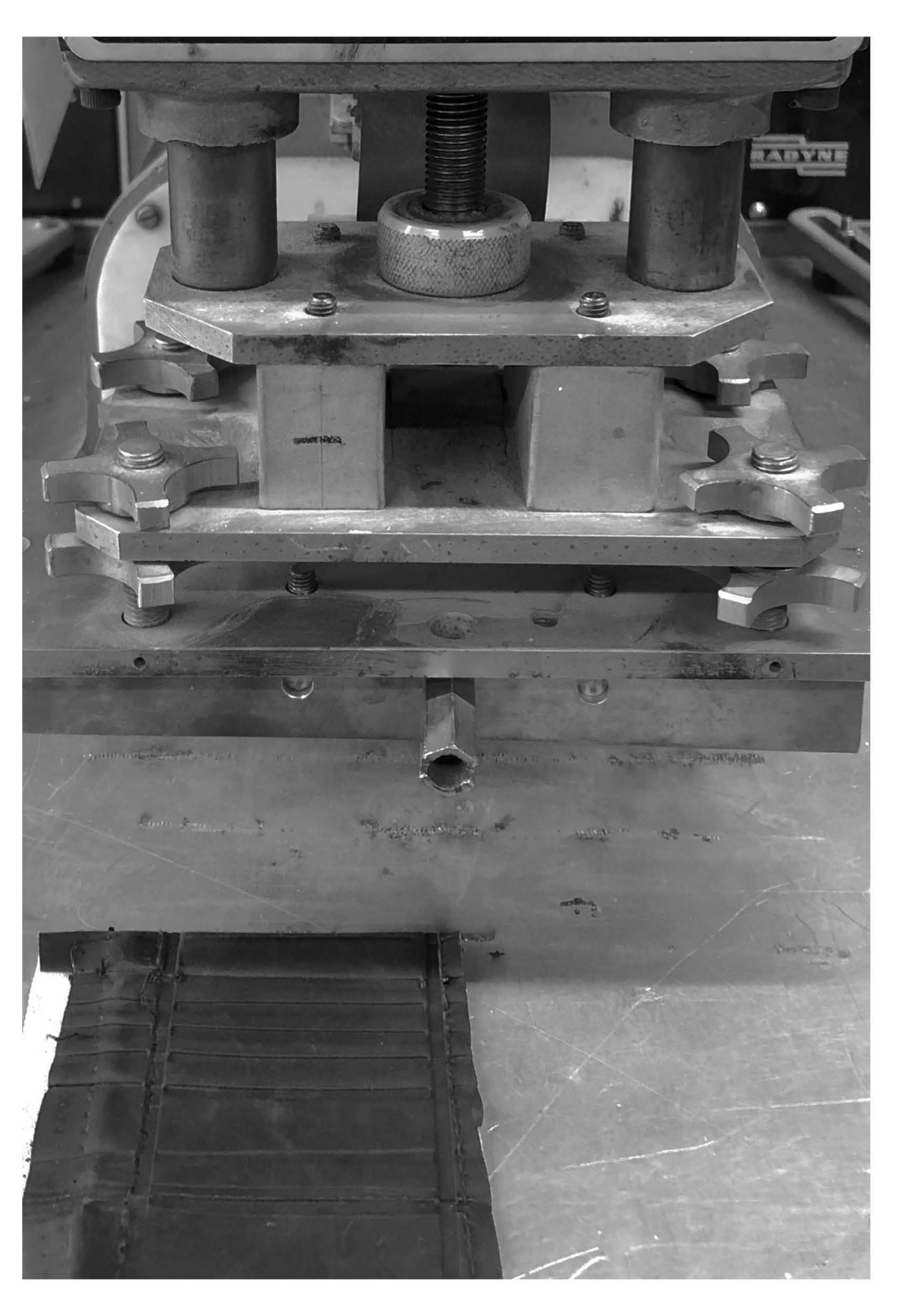
plastic bonding machine that melts together the two layers to bond them together leaving an embossed finish
