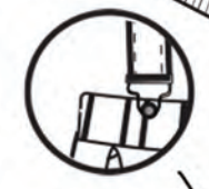
BRACE ATTACHMENT TO 2:1 RIBBED WAISTE
